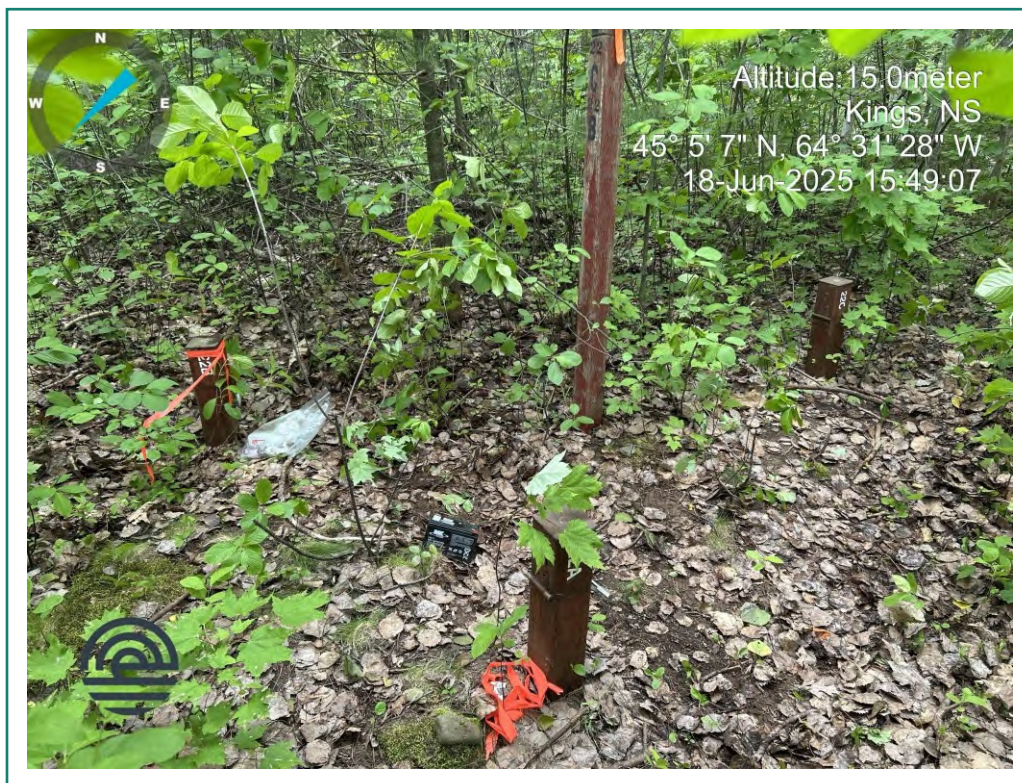
Photo 18: Monitoring Wells MW22A (center), MW22B (left), and MW22C (right).
